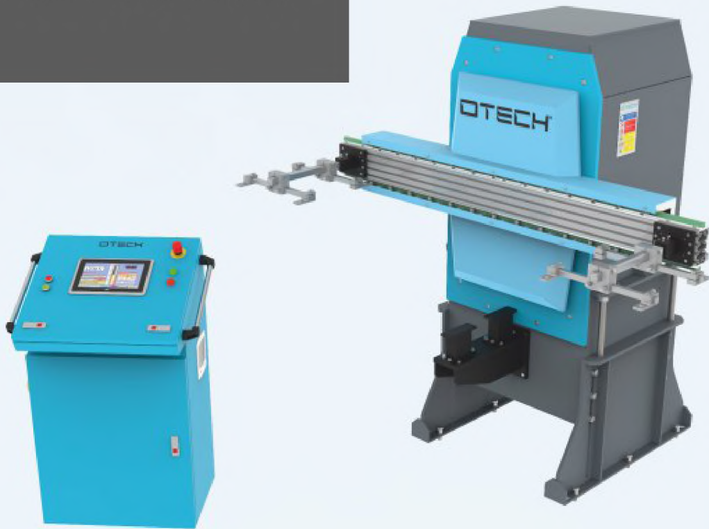
Transfer Robot Between Presses
